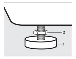
Using the spanner supplied turn counternut 2 in a clockwise direction.
